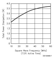
FIGURE 6. Power Dissipation vs Frequency
