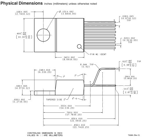
CONTROLLING DIMENSION IS INCH VALUES IN [ ] ARE MILLIMETERS
