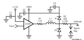
FIGURE 9. One Channel of the LM2439 with the Recommended Application Circuit
