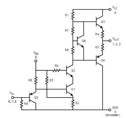
FIGURE 1. Simplified Schematic Diagram (One Channel)
