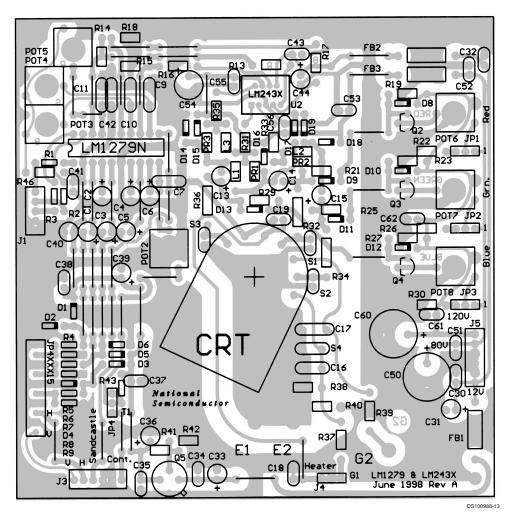
FIGURE 11. LM1279/243X Demo Board Layout
