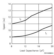
FIGURE 8. Speed vs Load Capacitance
