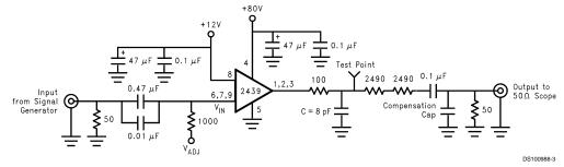
Note: 8 pF load includes parasitic capacitance.
